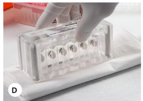
Figure 4. Separation of magnetic beads in tube format
