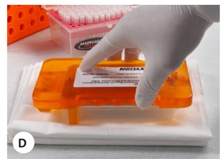
Figure 2. Separation of magnetic beads in microplate format
